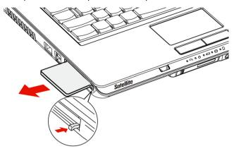
Figure 8-2 Removing the PC Card/ExpressCard
